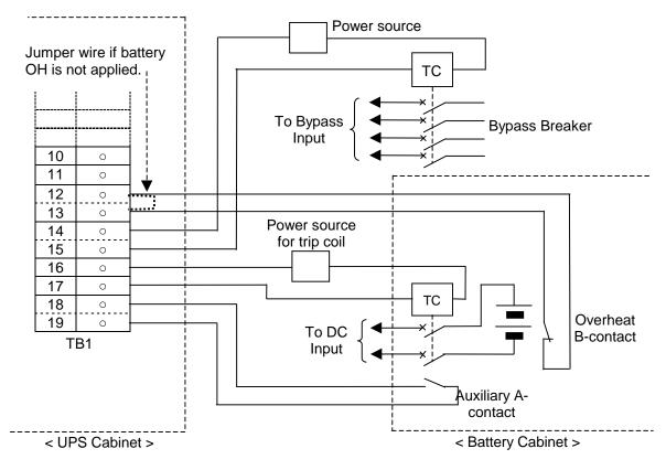
Figure 11 Connection among UPS, battery cabinet & bypass breaker.
